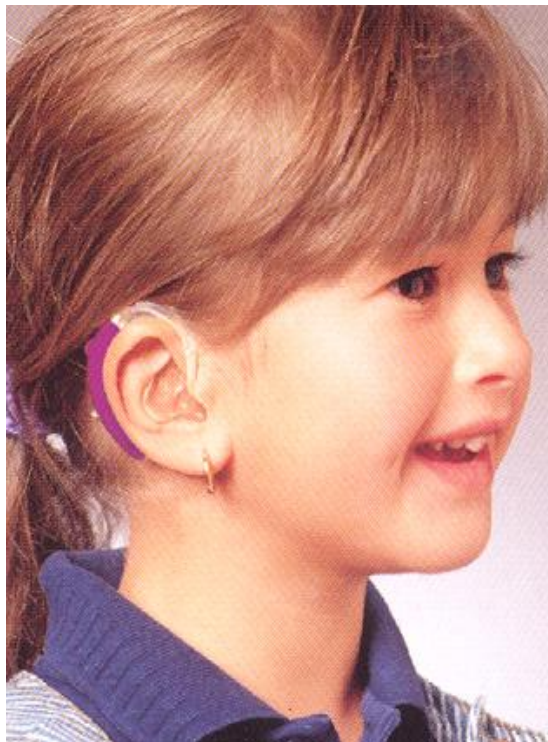
Fig 11. Behind the ear (BTE) hearing aid
